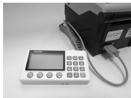
An example of optional keypad connection to the printer.
