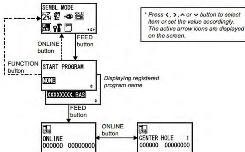
1. During Offline mode, press **FUNCTION** button to display the operational icon menu. Press arrow buttons to select SEMBL MODE.
