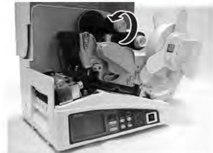
6. Remount the **print head** by turning the **head lock lever** clockwise until it latch on. The print head should lock into place firmly.
