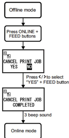
1. When the printer is Offline, pressing both the **ONLINE** and **FEED** buttons at the same time will switch the printer to CANCEL PRINT JOB mode. The menu for canceling the print job then appears.
