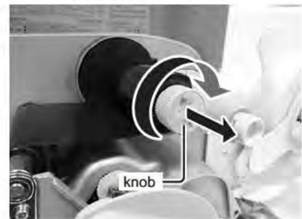
3. Remove the wound-up carbon ribbon from the **take-up spindle** in the direction of the arrow.
