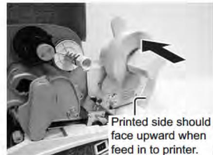
5. Attach the **roll media guide** back and make sure that the **roll media guide** pushes snugly against the media roll to prevent media drift during printing.
