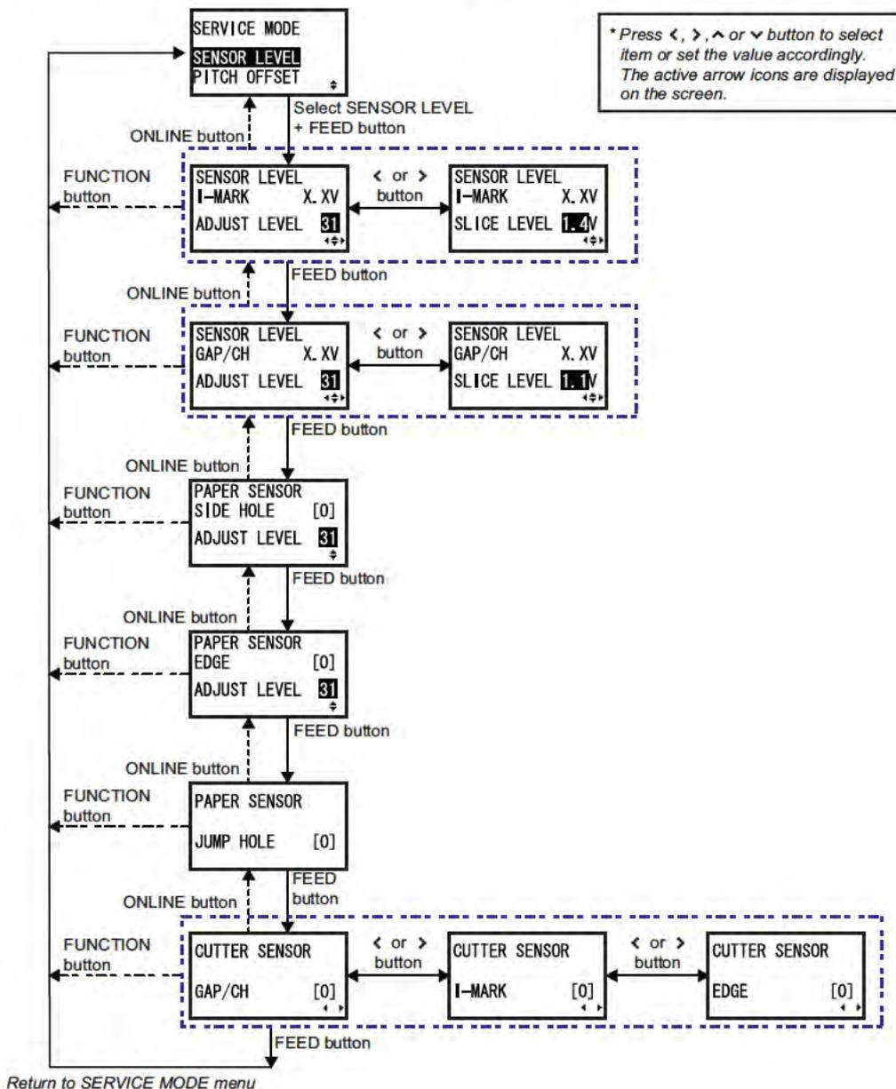
1. When SENSOR LEVEL is displayed, press the **FEED** button repeatedly will switch to the next setting options as shown above. To return to the previous setting option, press **ONLINE** button.
