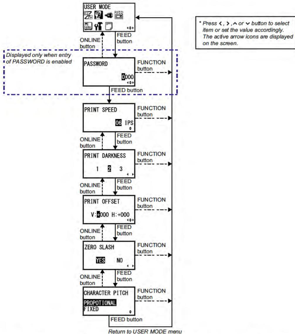
1. During Offline mode, press **FUNCTION** button to display the operational icon menu. Press **arrow** buttons to select USER MODE.
