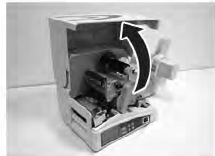
2. Remove the roll media guide by pressing the release tab with your thumb and index finger and pulling it out.
