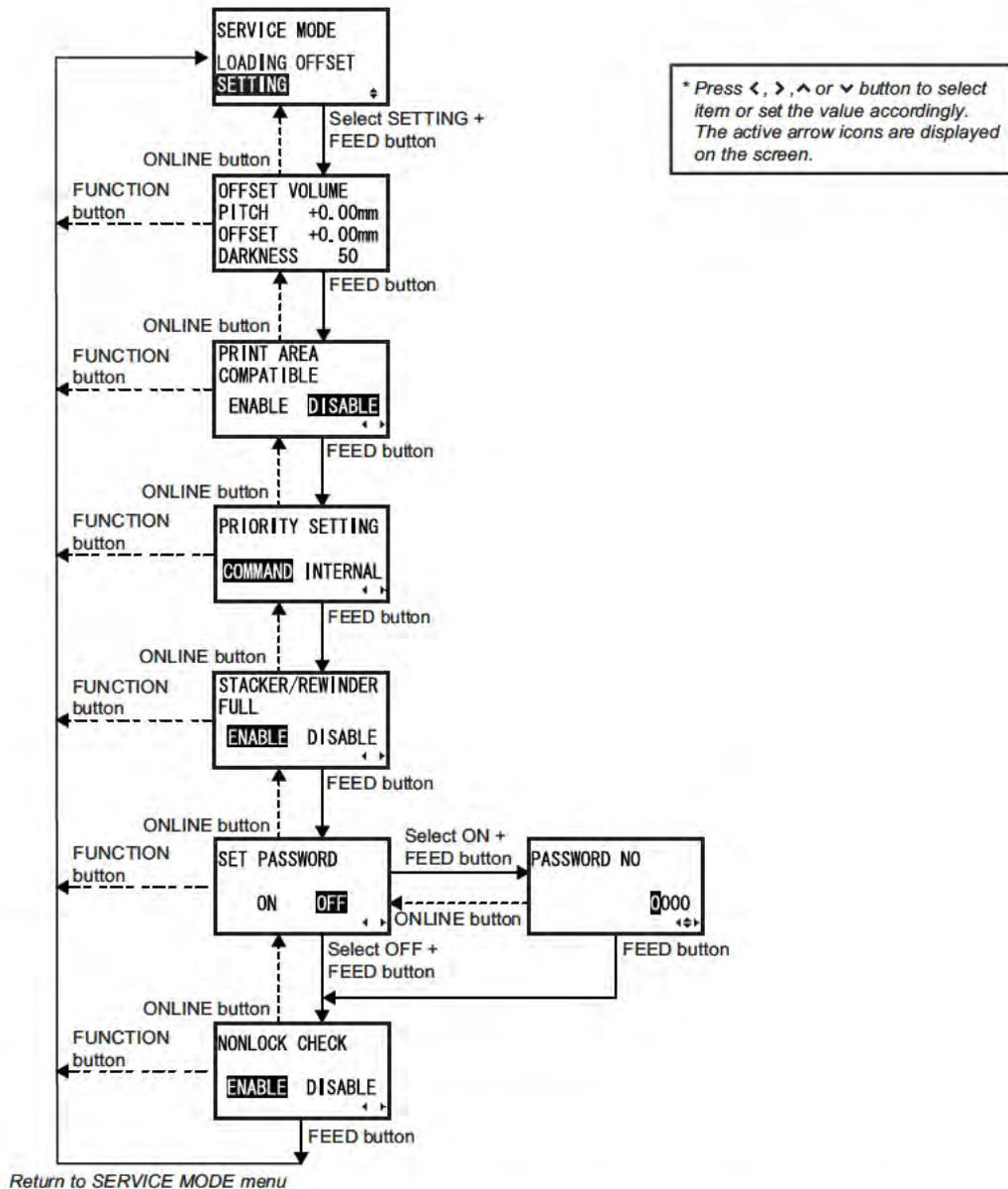
1. When OFFSET VOLUME is displayed, press the **FEED** button repeatedly will switch to the next setting options as shown above. To return to the previous setting option, press **ONLINE** button.
