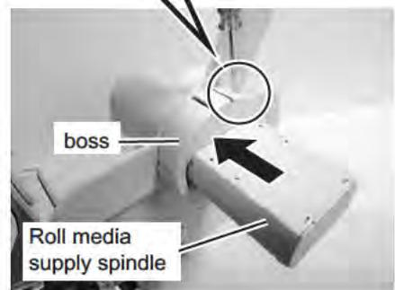
4. Load the media to the **roll media supply spindle**. Make sure the media leader is pull out from the bottom and the printed side is facing upwards. Push the roll firmly towards the end of the spindle.
