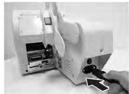
2. Insert the power plug into a AC power outlet.
