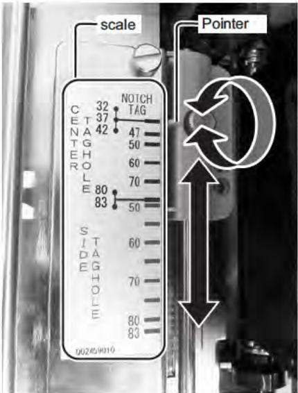
4. After adjusting the **Cutter sensor**, tighten the **Sensor adjustment thumbscrew** and close the **Cover**.
