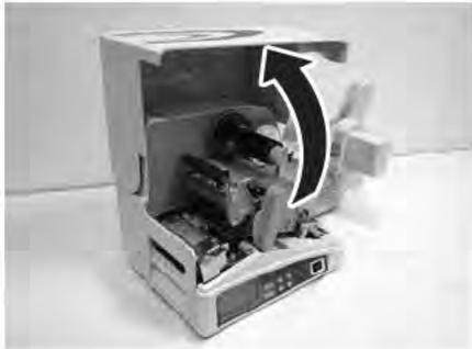
2. The purple **Cutter sensor assembly** is located in front of the **print head assembly**. Loosen the **Sensor adjustment thumbscrew** on the purple **Cutter sensor assembly**.
