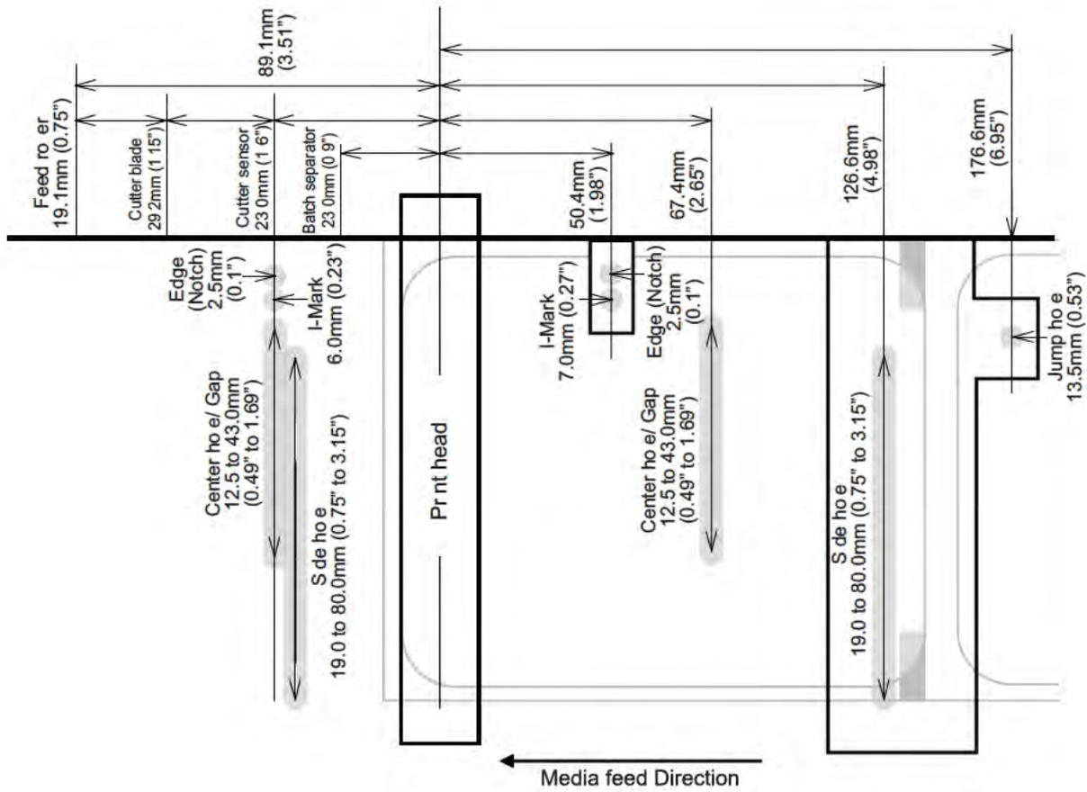
Only center hole sensor and Gap sensor are in common use. There is no interference among sensors shown above.
