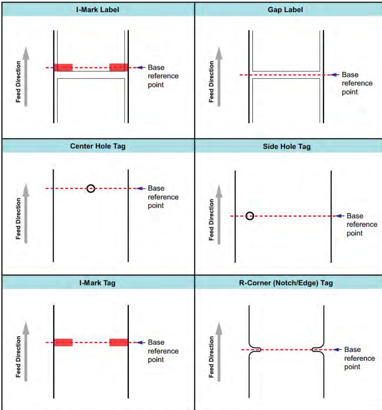
The center of each mark or hole is defined as the base reference point.
