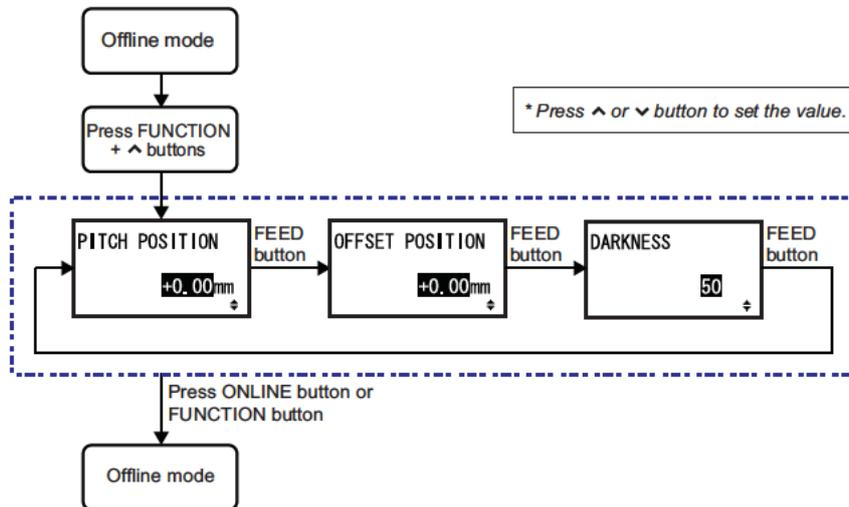
1. When the printer is Offline, pressing both the **FUNCTION** and **^** arrow buttons at the same time will switch the printer to Adjustment mode. The PITCH POSITION screen is displayed.
