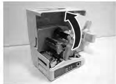
2. Turn the purple **head lock lever** counter clockwise to release it.
