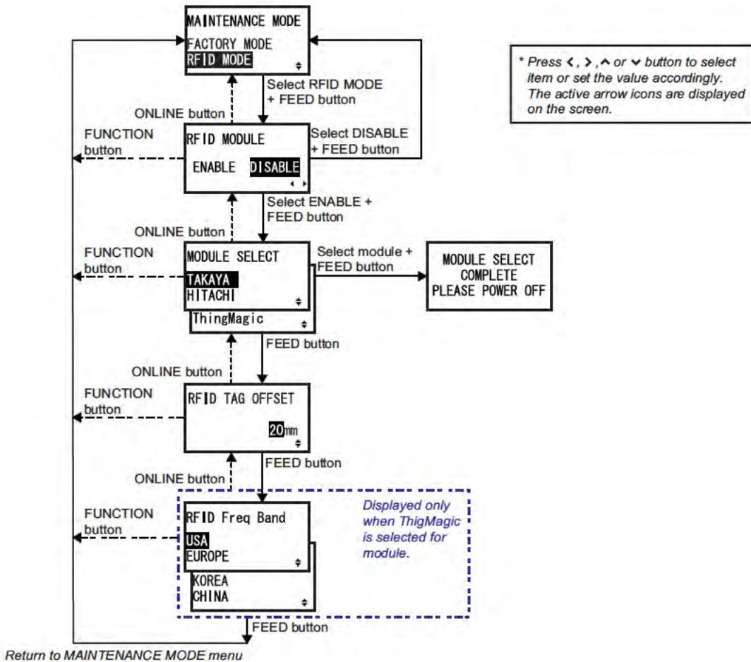
1. When MAINTENANCE MODE is displayed, press ^/v arrow buttons and then FEED button to enter to RFID MODE.
