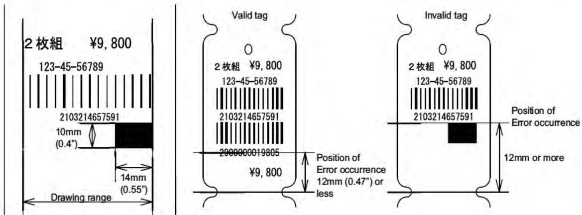
When the cutting motion is activated, an end mark will be printed regardless of position where an error occurred (within 12mm, 0.47").
