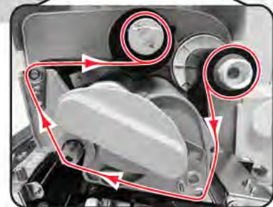
5. Then turn the **take-up spindle** several times in the direction of counter-clockwise to wind the ribbon around the **spindle**.
