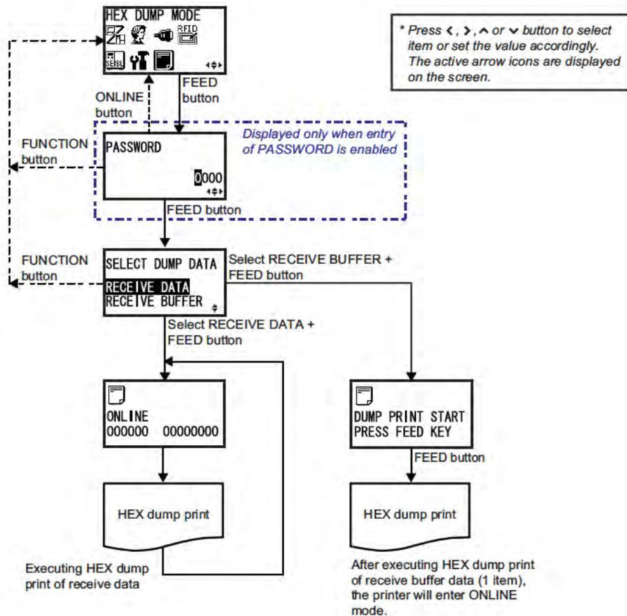
When HEX DUMP MODE is displayed, press the **FEED** button to enter to HEX Dump mode.
