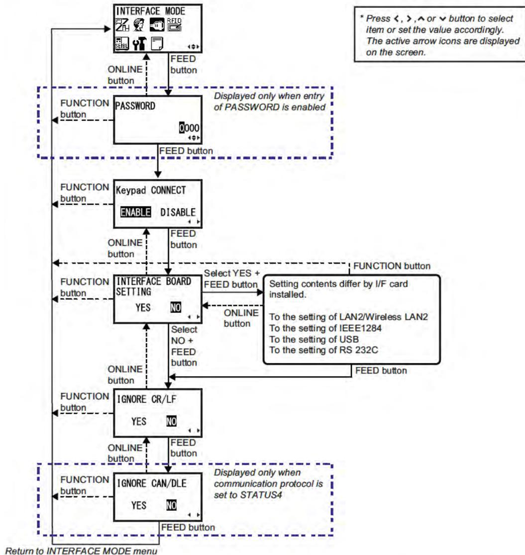
1. During Offline mode, press **FUNCTION** button to display the operational icon menu. Press **arrow** buttons to select INTERFACE MODE.
