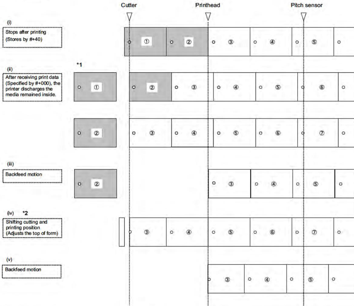
\*1. For the printer without cutting motion, ① will be discharged without being cut, but ② will be cut and discharged.
