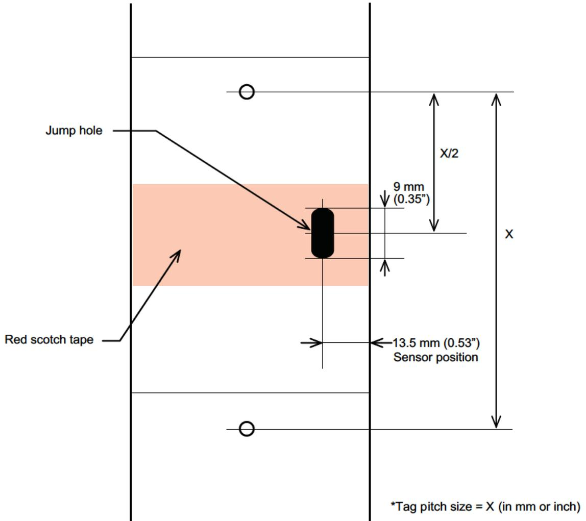
The width of jump-hole tag must be between 37mm (1.5") and 80mm (3.15"), and the pitch size must be 40mm (1.6") or more. Also, the center of jump-hole must be at "Vertical position = Pitch (X)/2 in mm or inches, Horizontal position = 13.5mm (0.53)".
