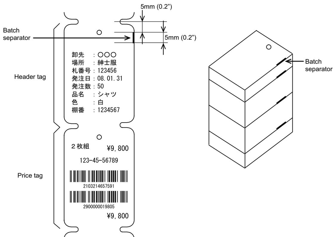
The batch separator is available only when being specified by the online command (ESC I1). When more than two tags are specified for printing, only the first tag will carry the batch separator.
