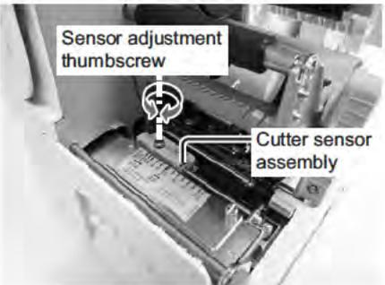
3. Slide the **Cutter sensor assembly** and align the **pointer** on the **Cutter Sensor Assembly** to the position of the tag registration mark using the **scale**.
