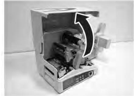
2. Turn the purple **knob** of the **ribbon take-up spindle** in counter clockwise direction and then pull outward. The **ribbon take-up spindle** is released and the wound-up carbon ribbon is loosen.
