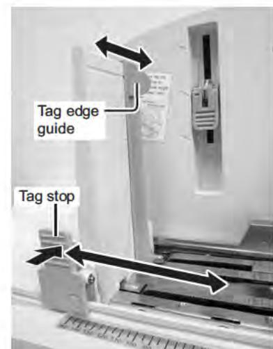
6. Send the print job to the printer and let it cut and stack a few tags. The temporarily stop the printer by pressing the **ONLINE** button and check to make sure the tags are being stacked under the **Tag Hold Down** and that the **Tag Stop** and **Tag Edge Guide** are properly set.
